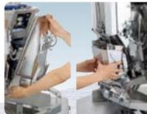
Unitization of actuator and feeder Easily removable and attachable buckets
